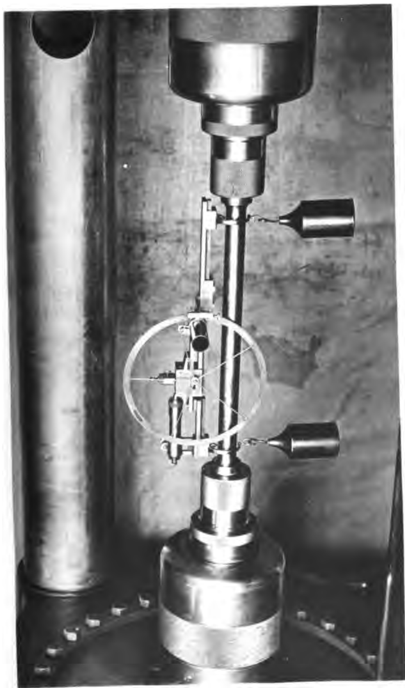
NO. 11. DIAL EXTENSOMETER, WITH SCREW MICROMETER.
